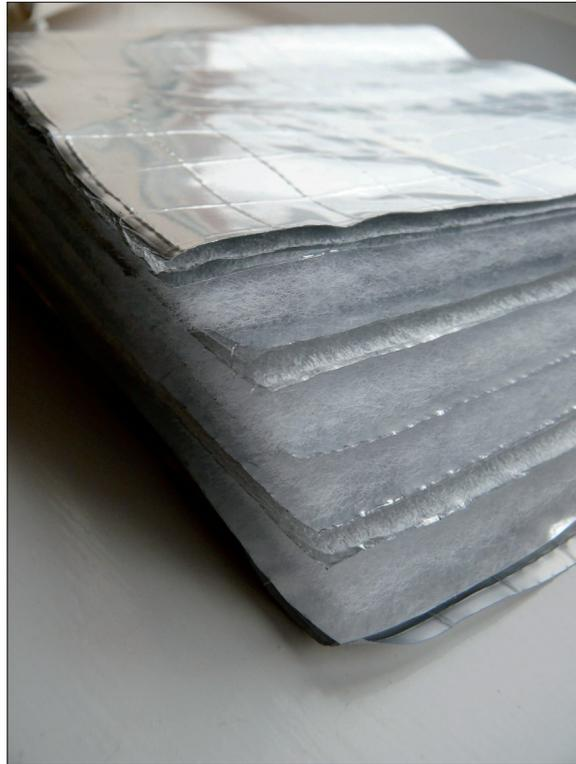
1.2 YBS self-adhesive foil-tape (75 mm) is used to seal overlaps, enabling the product to act as a vapour control layer.
